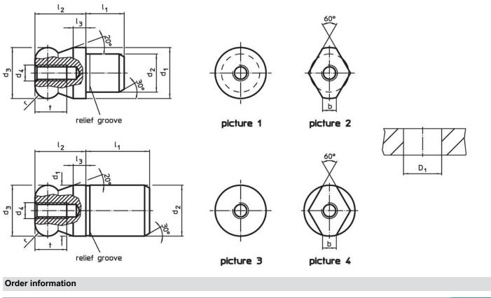
Dimensions Location hole Art. No. D d<sub>3</sub> b d₁ d<sub>2</sub> d₄ h l<sub>2</sub> I<sub>3</sub> t r H7 g6 n6 -0.01 -0.05 [g] [mm] [mm] with ball end flattened - picture 2, Stainless steel 6 М3 6 8 2 6 2 2 6 3.2 22630.0448 8 8
