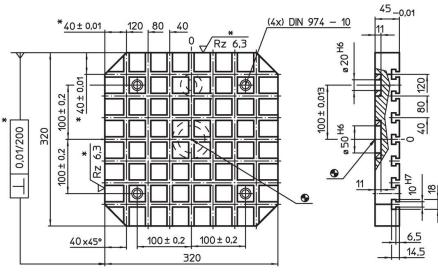
$^{\ast}$  These tolerances are valid only for optional exterior stop type. Slot spacing 40  $\pm0.01.$
