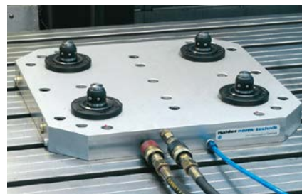
Machine table: Base plate with 4 connecting elements
