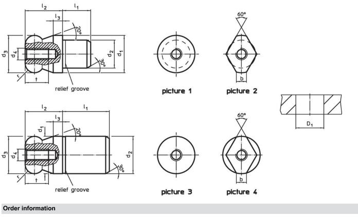
Dimensions Location hole Art. No.  $D_1$ d₁  $d_3$  $d_2$ d₄ l<sub>2</sub> I<sub>1</sub> l<sub>3</sub> t r H7 g6 n6 -0.01 -0.05 [mm] [mm] [g] ball end round ball - picture 1, Tool steel 22630.0312 12 8 12 M4 8 12 3 8 3 8 11
