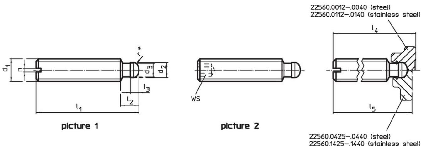
\* to ease assembly the DIN 6332 specification has been completed by r
