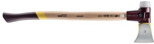
Splitting axe and soft-face mallet in one, axe blade drop-forged and hardened, ground and polished, solid handle-protection sleeve, insert made of superplastic, KWF-certificated, all parts are replaceabl
